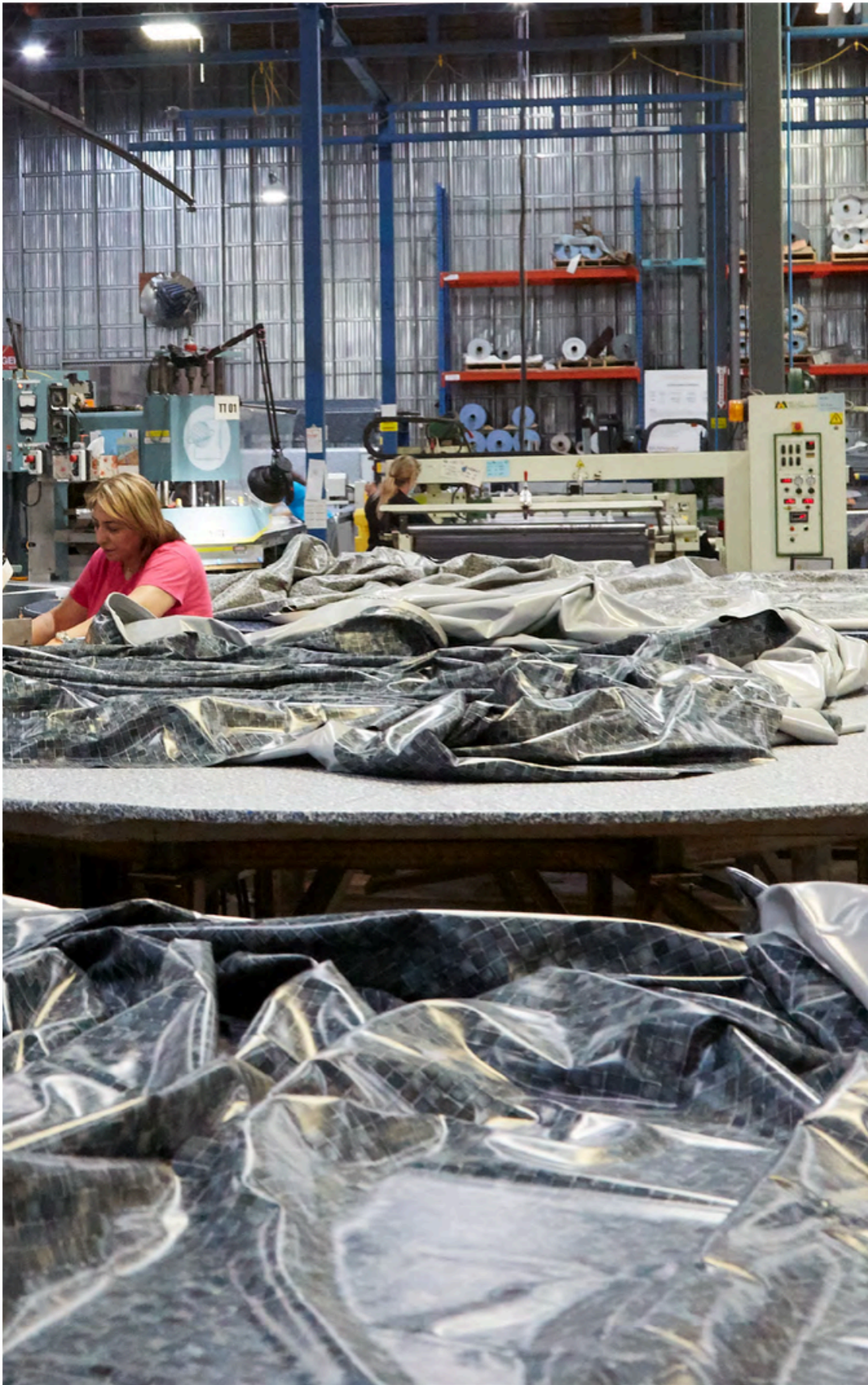
Sealing the liner sections with high intensity heat.
