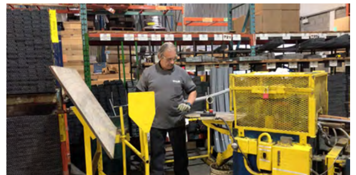
Profiling of structural components.
