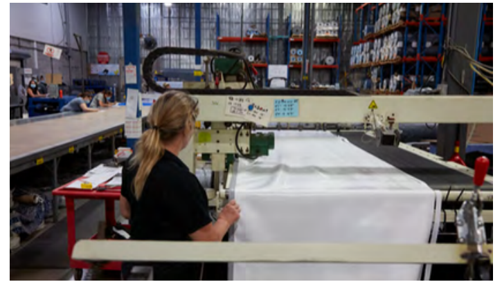
Welding the hanging profile to the vinyl wall.
